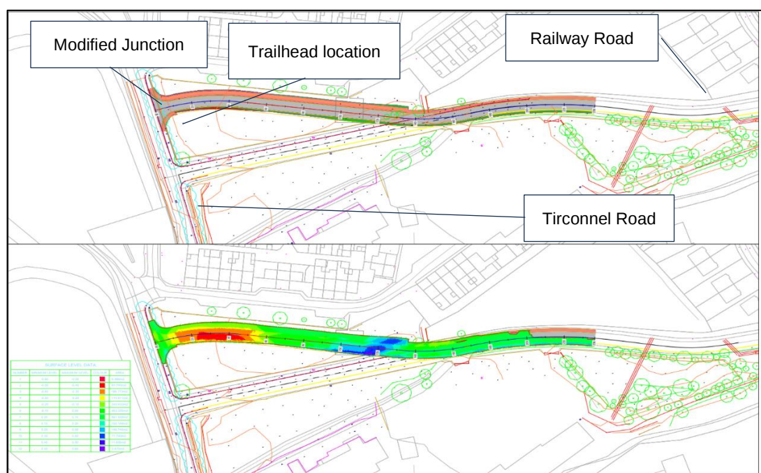
Figure 4-4 - Donegal Trailhead Cut & Fill Analysis
